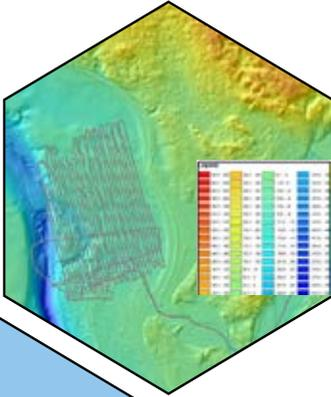
Seamless map of coastline and seabed generated using a combination of Lidar, and remote sensing techniques including multibeam sonar. Image: GEUS
