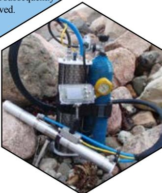
Proof of concept underwater device to non destructively assess the state of preservation of wood in situ. Image: AKUT
